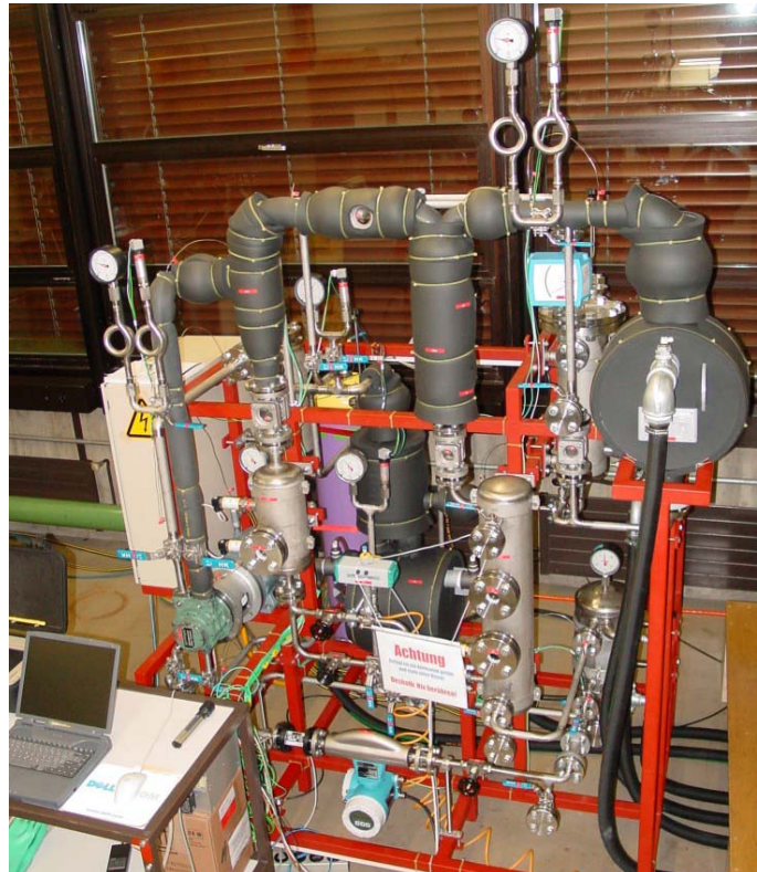
Figure 8-23 Functional demonstrator of a brine/water heat pump with ammonia as a refrigerant and an open rotary vane compressor [Kopp 2001]
