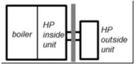
• PRODUCT 2 : As an un-integrated combination heater : A thermally driven heat pump coupled with a separated auxiliary boiler.
