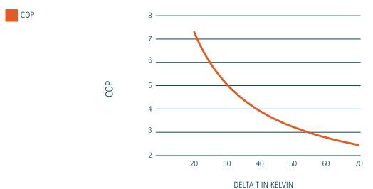
The coefficient of performance is determined under standard conditions in a laboratory. This standardized approach allows the comparison of different heat pumps with regards to their efficiency. Measurements are based on standard <u>EN14511</u>.
