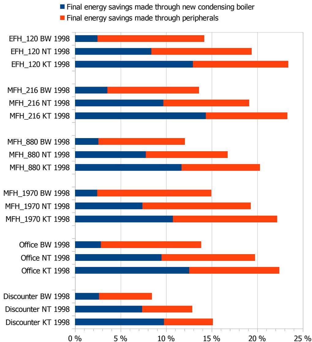
figure 1: fuel savings made in 6 buildings through replacing aging constant-temperature (KT), low-temperature (NT) and condensing boilers (BW) with a new condensing boiler; differentiated according to boiler and peripheral
