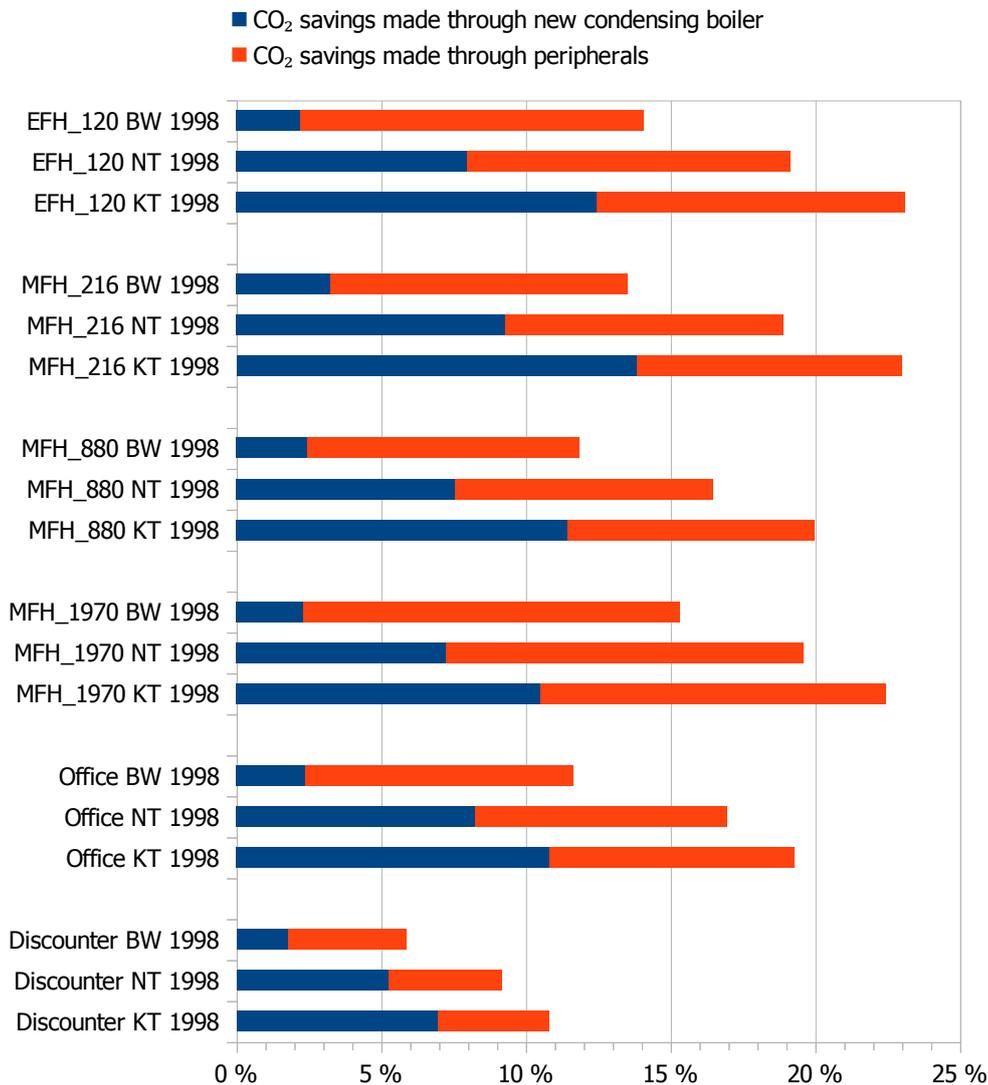
figure 2: CO<sub>2</sub>eq savings gained in 6 buildings by replacement of aging constant-temperature (KT), low-temperature (NT) and condensing boilers (BW) with new condensing boilers; differentiated according to boiler and peripherals
