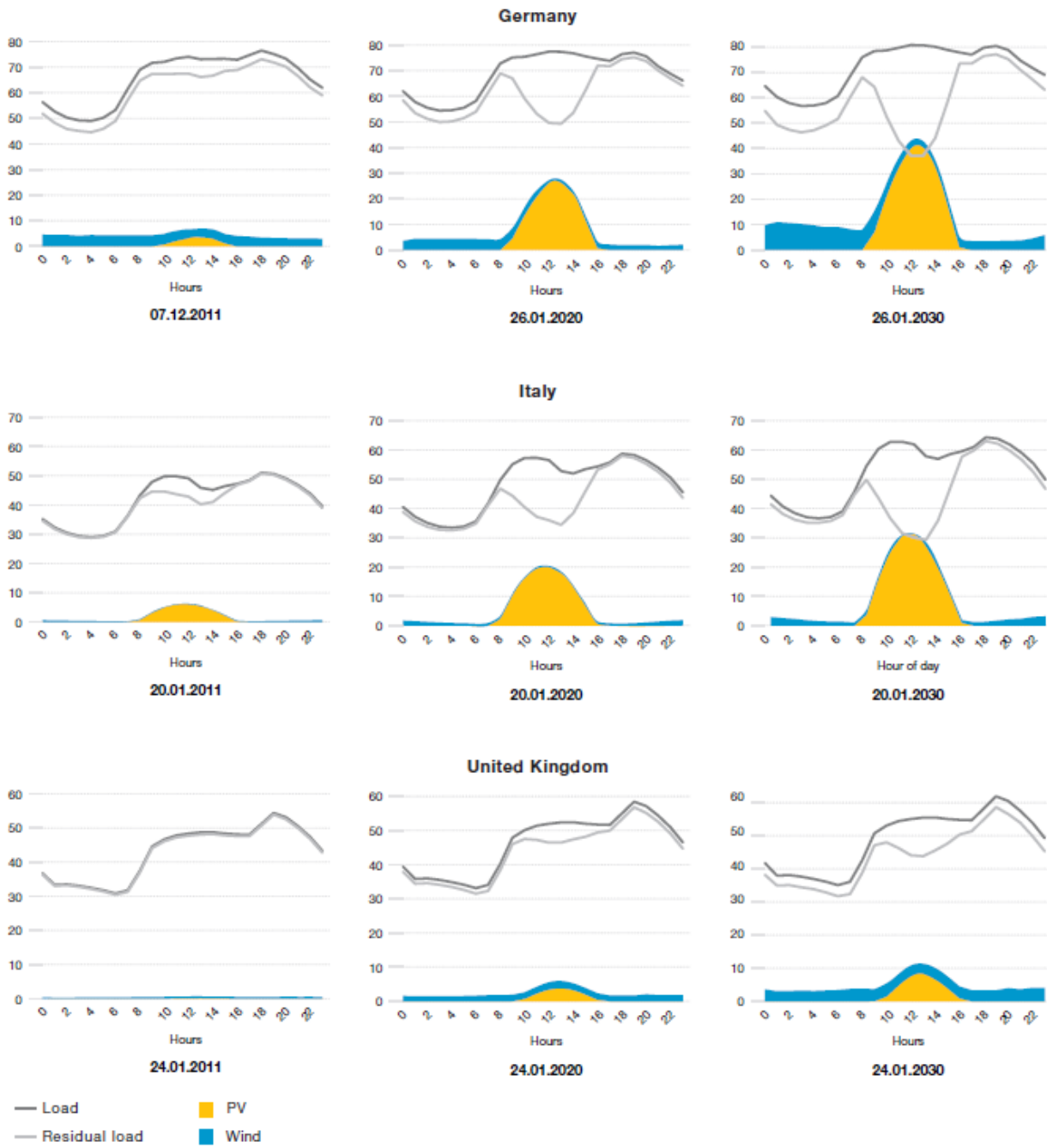
Figure 1 – The evolution of the residual peak load in Germany, Italy and the UK (2011, 2020 and 2030)
